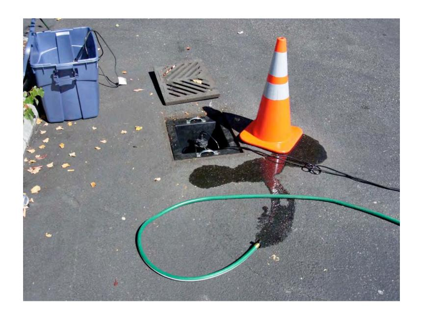
Figure 2 – View of Storm Drain and Water Effluent Collection Device
